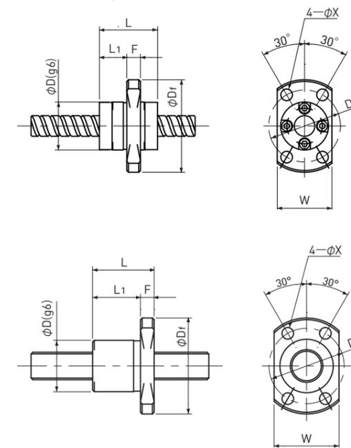
Type-2 : End-cap type (Ball Screw Nut)
