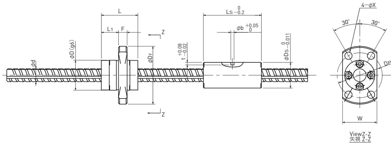
Type-2 : End-cap type (Ball Screw Nut)
