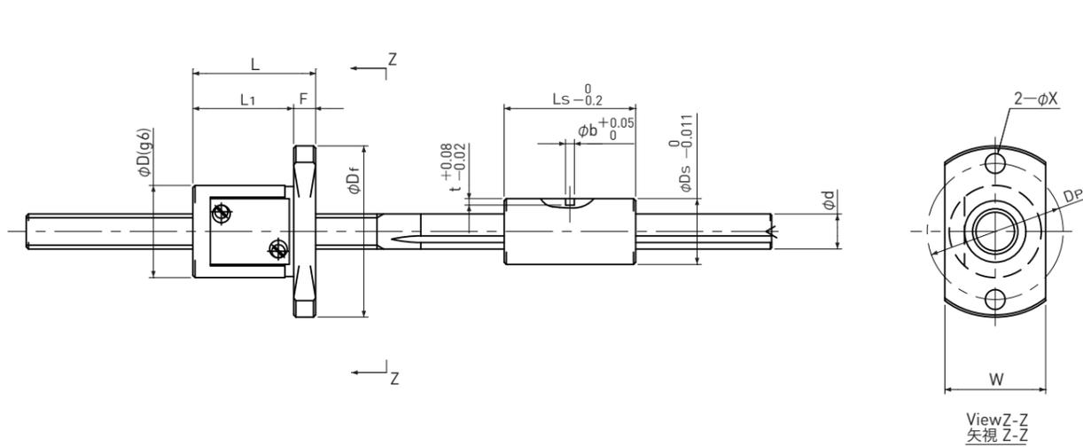
Type-1 : Return-plate type (Ball Screw Nut)
