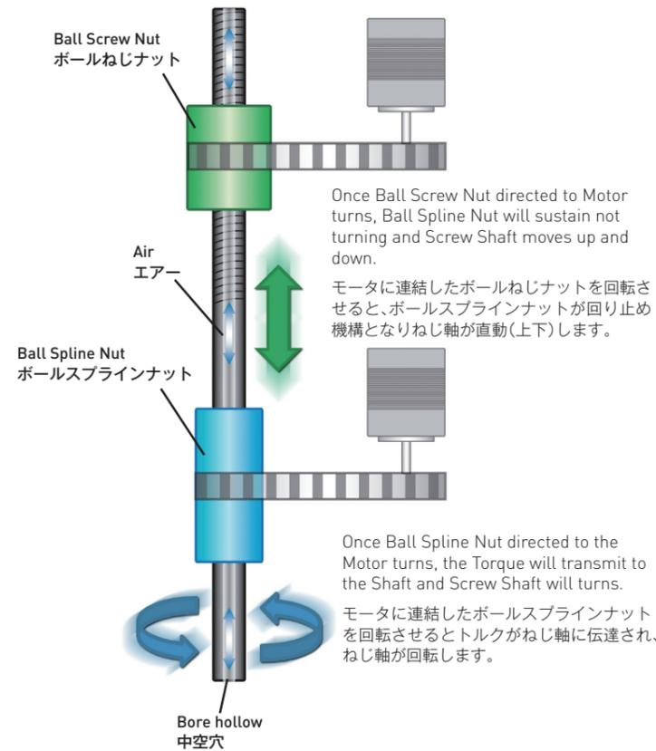
Bore hollow can be multi uses. For example vacuum and blow function.
