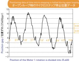
Position of the Motor 1 rotation is divided into 25,600 and the stop position of a Motor is formed into database モータ1回転を25600分割してモータの停止位置を
